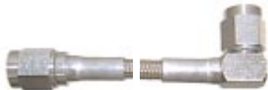
-3 an Female Swivel straight to -3 Female Swivel 90° - size 3 Hose
