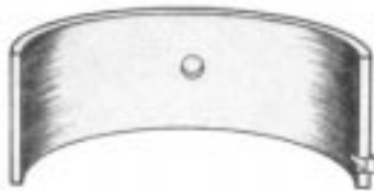
Figure 3: Wide wear pattern
