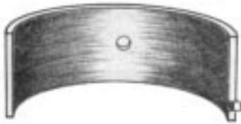
Figure 2: Narrow wear pattern
